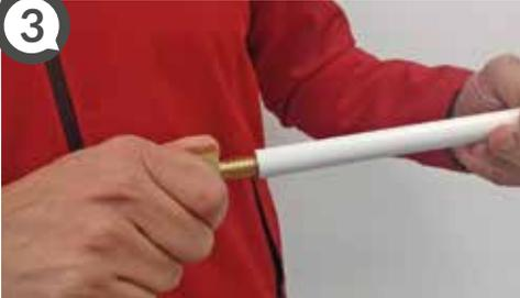
Thread the fitting into the pipe to the end.
