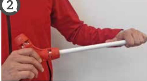
Calibrate and bevel the pipe.
